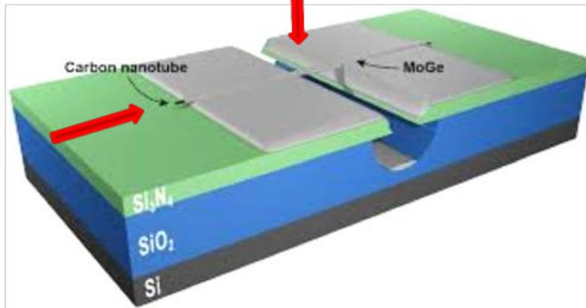
**Fabrication: molecular templating technique**
