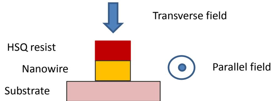
Measurements are done in dilution refrigerator with well-filtered lines in transverse and parallel magnetic fields
